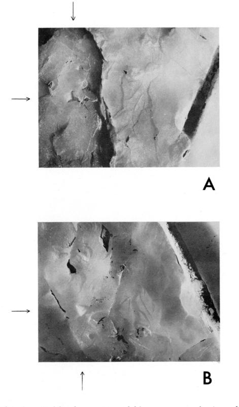
Plate 1. Models of a specimen of fybrous gypsum, showing sedimentary structures; A, upper surface; B, lower surface.
